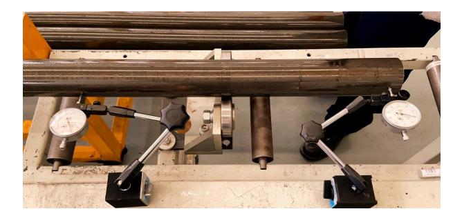
To ensure that your drill rods spin straight and to minimise rod vibration (rod slap), we apply 2 test methods.
