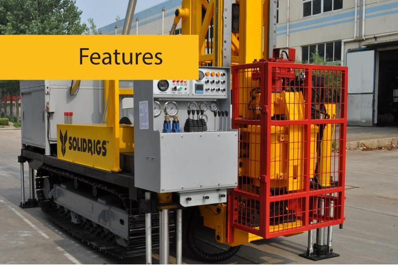
The SRD series is one of the most versatile and cost effective drill rigs in today's market. A heavy duty drill rig that has been designed specifically for drilling deep holes across a wide range of drilling applications such as mineral exploration, directional drilling and geotechnical drilling. It has being designed to reach depths of up to 2,500m NQ, 1,600m HQ and 1,000m PQ.
