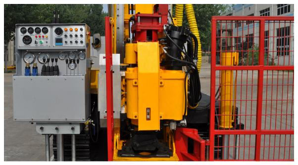
For safety, the rod guards are fitted with sensors which stops the drill head's rotoation when it is opened during operation.
